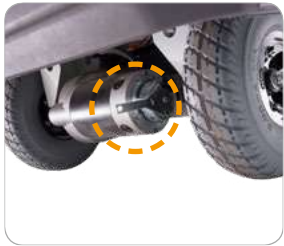
Manual switching lever This lever enables to switch to manual drive at narrow spaces or while battery is discharging.
