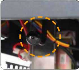
Manual switching lever on the control panel Enabling driving for narrow space or when the battery is discharged.
