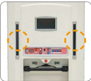
Front touch sensor (optional) Reducing the speed in emergency.
